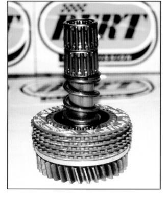
Assemble clutch with dummy shaft.
